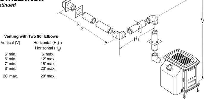
Figure 29 - Horizontal Termination Configuration for Rigid Venting Using Two 90° Elbows with Termination at 90° with Stove
